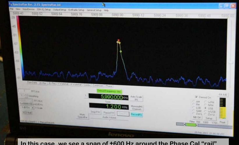
In this case, we see a span of ±600 Hz around the Phase Cal "rail". The Resolution Bandwidth (RBW) is 0.85 Hz and the screen is showing a 40 dB amplitude range.
